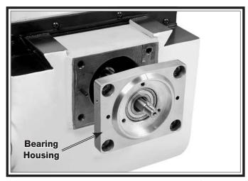
Figure 63. Removing the bearing housing from the cross leadscrew.
